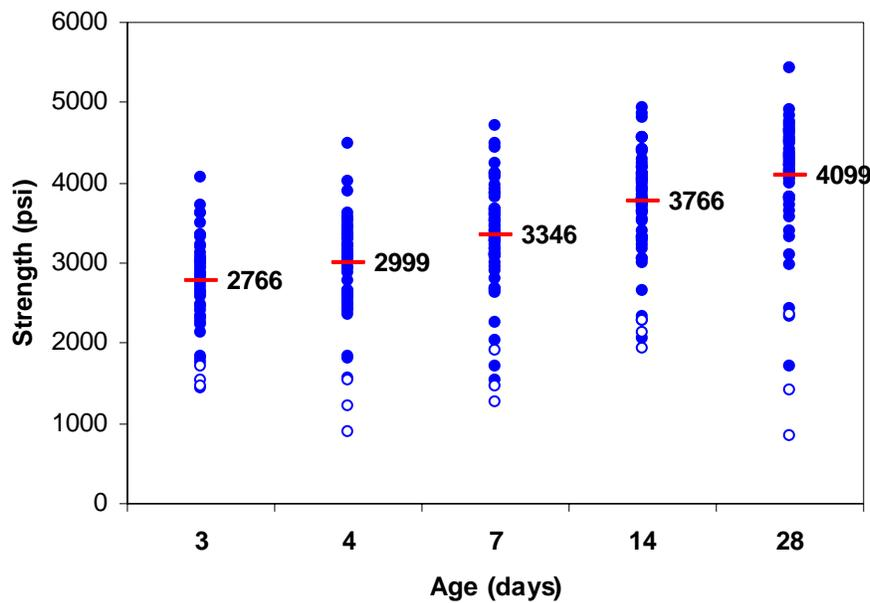
**FIGURE 7 Individual cylinder strengths.**
