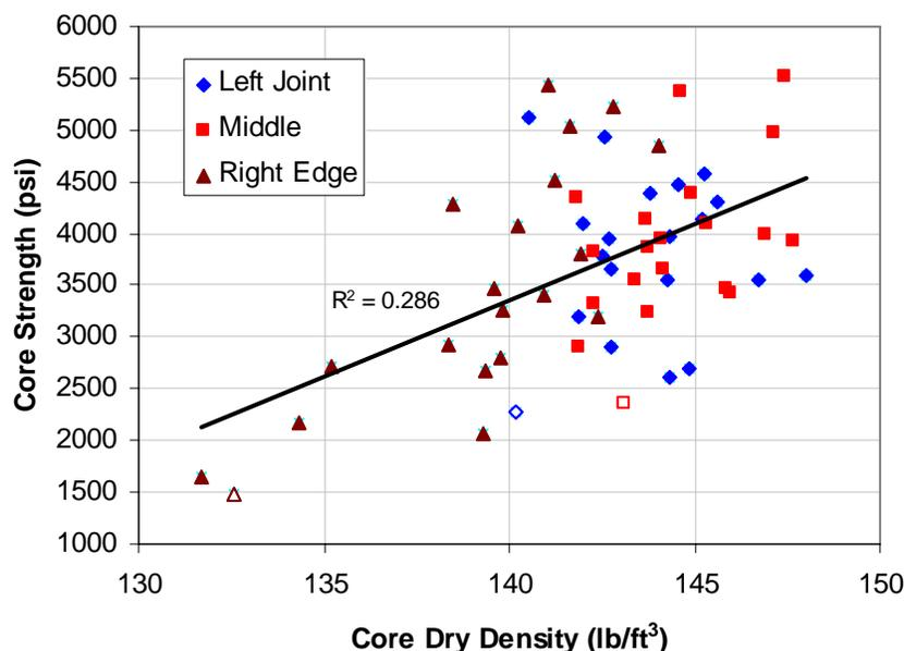
**FIGURE 8 Core Strength vs. Core Dry Density.**
