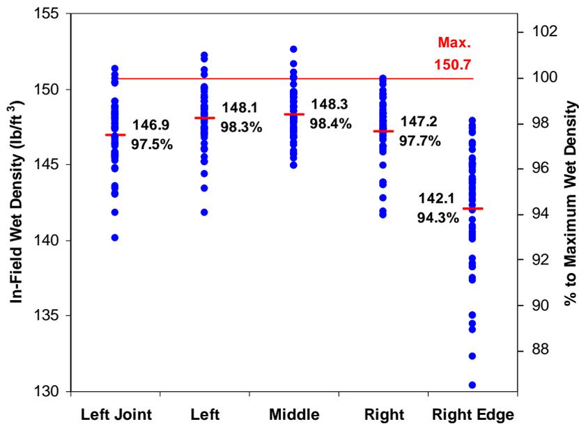
**FIGURE 4 Individual wet density readings by nuclear gage.**
