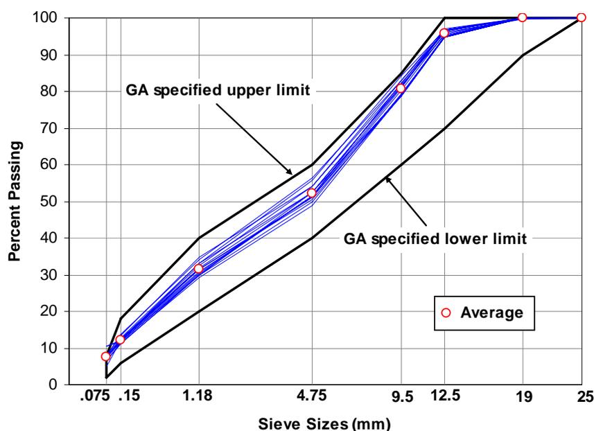
**FIGURE 3 Gradation of RCC mixes.**
