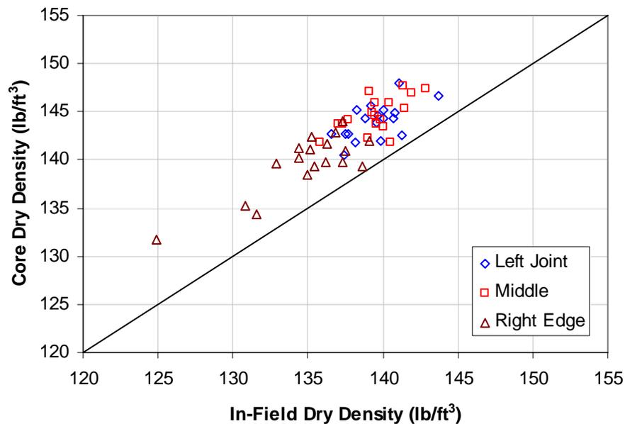
**FIGURE 6 Core density vs. In-Field density.**
