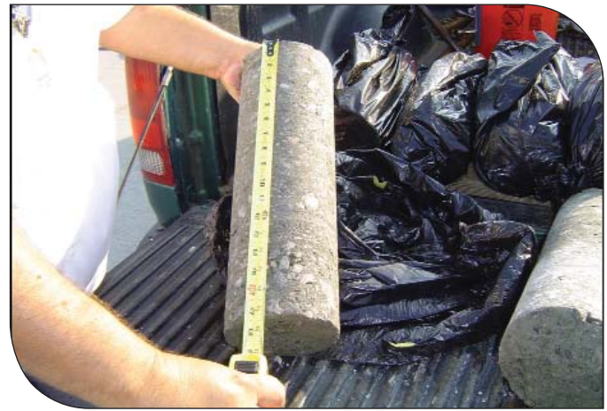
Quality control check using pavement cores after 7 days.
