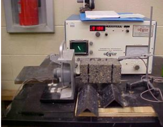
Figure 11. Sonometer testing device.
