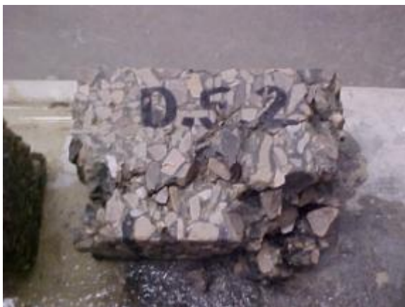
Figure 12. Dam series specimen number 20 at 236 cycles.
