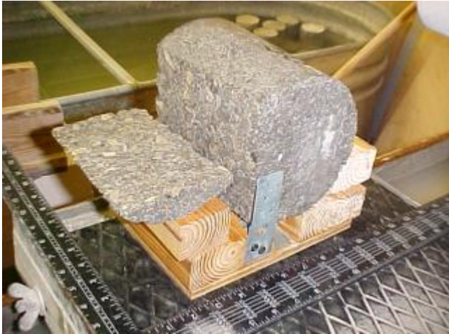
Figure 9. Photo of jigs with one side sawn of an RCC specimen.
