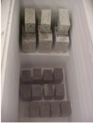
Figure 10. Prisms in freezer before testing.
