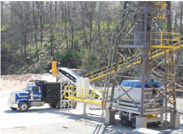
Figure 6. Twin shaft horizontal mixer—batch type.
