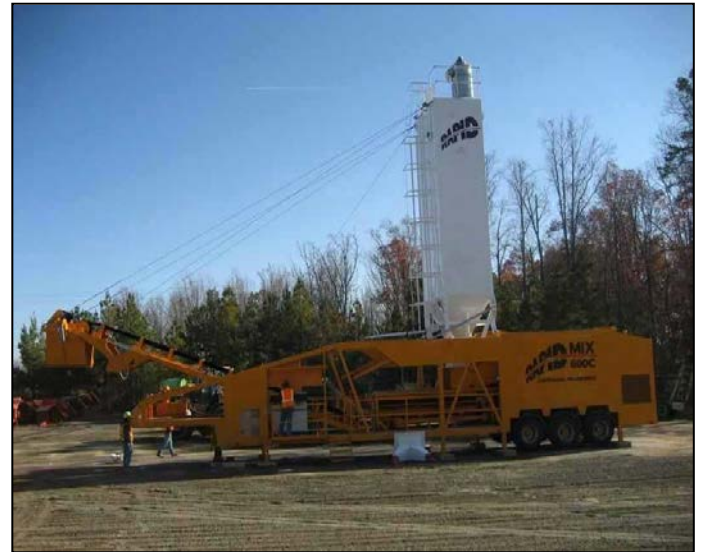
Figure 7. Twin shaft horizontal mixer—continuous type.
