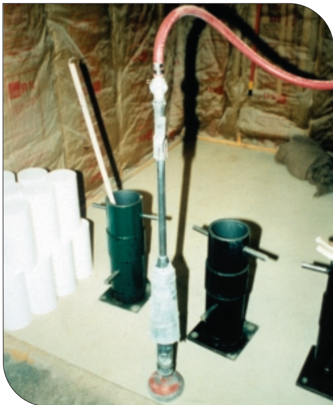
Figure 7. Preparation of RCC using a pneumatic tamper.
