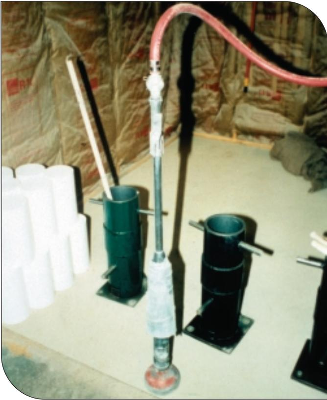
**Figure 7. Preparation of RCC using a pneumatic tamper.**
