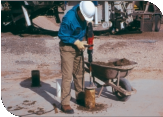
Figure 6. Vibrating hammer used to prepare RCC cylinder (ASTM C 1435).
